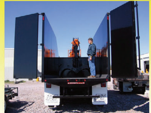
40-45 cubic yard heavy duty trash dump body
